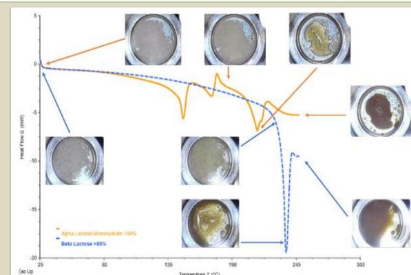
Figure 2: Thermogram overlay between  $\alpha$ -lactose monohydrate and  $\beta$ -lactose with optical images at different stages
