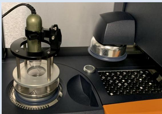
Figure 1: DSC-hyphenated with microscope imaging.
